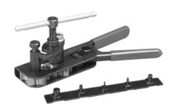
FLARING CAPACITY: %6", ¼", %6", ½", %1", ½", and %1" O.D. for single flares, and up to ½" O.D. for double flares. Can be used with copper, aluminum, brass, bundyweld and steel tubing.
