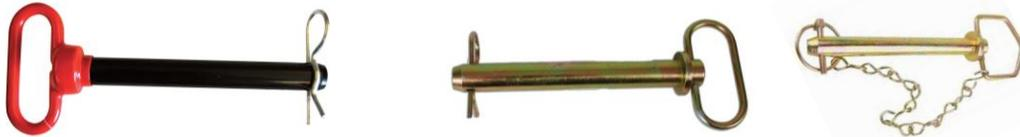
The towed implement will have a forked tongue with holes that slip over the drawbar and is held in place with a Hitch Pin. These come in a wide variety of sizes and are held in place with a linch pin.
