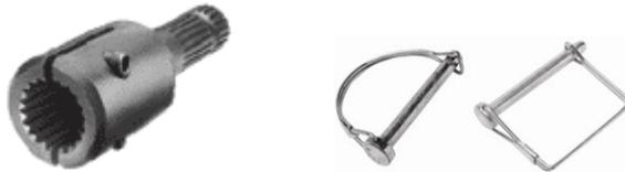
The Power Take Off is a splined shaft protruding from the rear axle of the tractor. It is used to drive the moving parts of implements such as rotary mowers by sliding the splined shaft into a splined coupling on the implement. When the tractor and implement are of different categories a PTO Adapter is used to mate the different size shaft and coupling and is held in place with a PTO lock pin.
